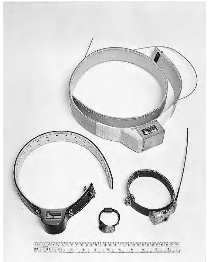
Figure 2.3 Radio collars. A variety of radio collars have been developed to use with mammals of different sizes. The collar, battery, and transmitter should not exceed about 10% of the weight of the animal. Thus, with constraints on collar size in smaller mammals, there are often limitations on the size of the battery and, consequently, on both the length of time the transmitter will be functional and the distance over which the signal can be detected.
